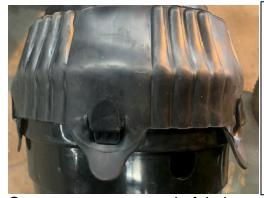
Pull on rubber tabs to release them from the plastic shroud and pull the rubber cover back. Grease zerks with 2 pumps as shown. Remember to grease all three cross bearings. The zerks are on the caps
