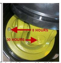
Once a year separate shaft halves and lube sliding parts with chain lube or white lithium grease.
